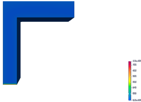
Figure 10: A sharp bend's temperature distribution along the symmetry plane.
